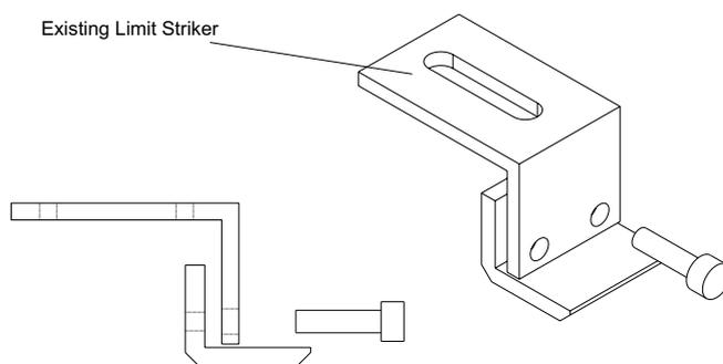
Drill 2 holes in existing limit striker and fit new limit dog with M4 screws
